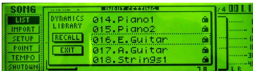
Select "016. E. Guitar" and press the [ENTER] key. You now have a dynamics processor (in this case, a compressor) applied to your guitar.
