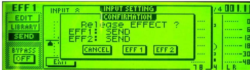
What this is saying is "You are going to use one of the effect processors as an insert to generate the guitar effects. Which one do you want to use and is that okay?" Use the cursor keys to select "EFF 1" and press the [ENTER] button. Realize that when we are done recording the guitar with effects we will be able to place that effect back as a send effect (send for every input and track).
