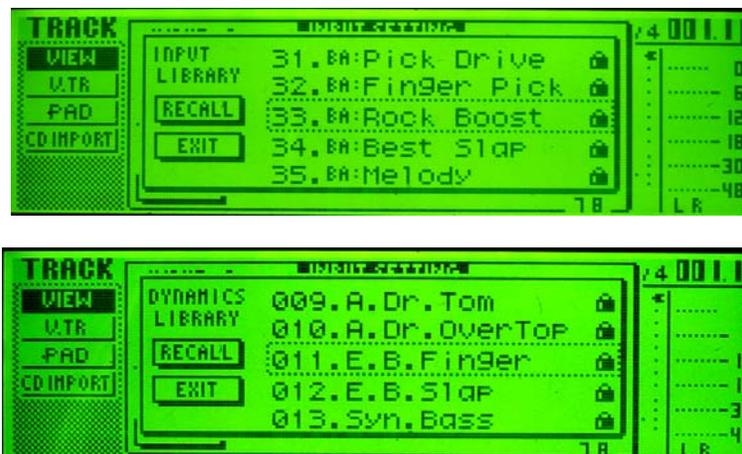
For acoustic bassists, the same idea as above with acoustic guitar considerations can be followed. If you have a bridge pickup, simply plug into channel 8 Hi-Z. If you are using a microphone only plug into channel inputs 1 or 2. There are no acoustic bass effect library parameters per se, but effect "BA:32 Finger Pick" gives a nice meaty, warm sound with a good attack. You can always bypass the input effects as well and
